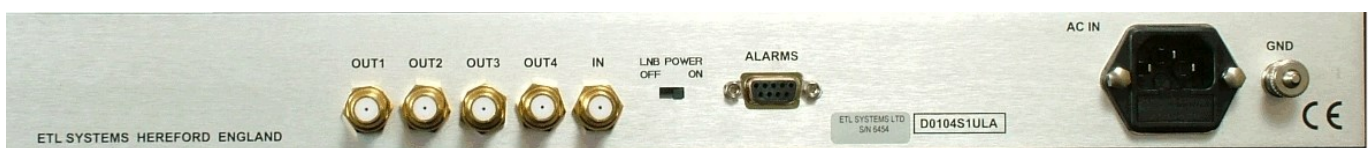
Rear view of LD Series Splitter showing switchable LNB Powering
